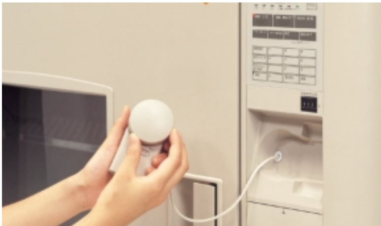
Jog dial for fine depressurization control
